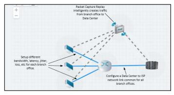
Packet Capture files can be large and complex making it difficult to identify application flows to replay. NE-ONE automatically analyzes and displays application flows, conversations between clients and servers, making it easy to select from the web GUI.
