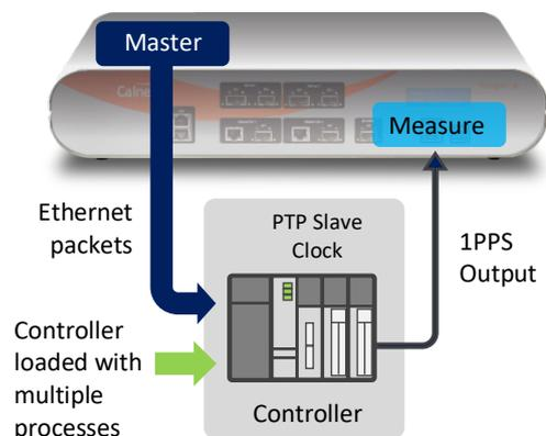
The maximum Time Error for the system is the combination of the worst-case error of the two scenarios.
