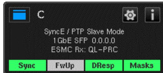
The full channel status, including the negotiated parameters can be displayed by pressing the **i** button.
