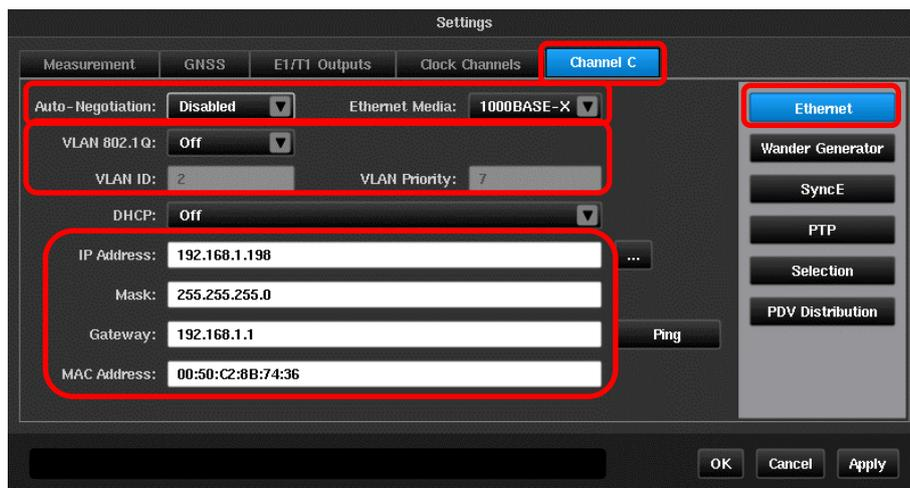
Ensure that the physical media properties match the properties of the port being connected to. Any required VLAN configuration should be entered. If a DHCP server is not being used then the IP properties should be manually entered.
