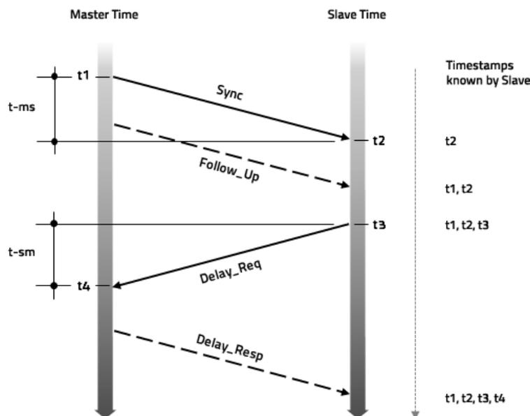
Once the Slave knows the timing of t1, t2, t3, and t4, it can calculate the mean propagation delay (Tmpd) of the messages path and slave clock offset. This can be calculated by:
