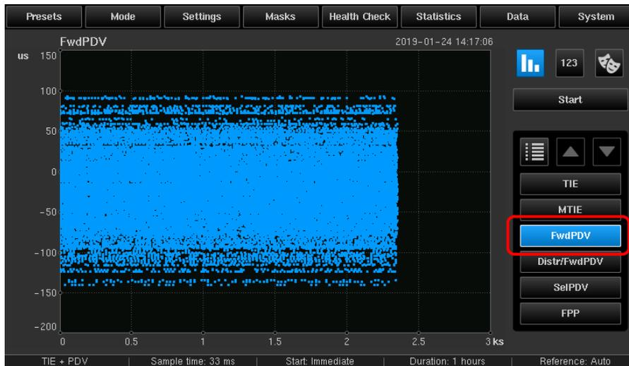
**NOTE:** Sentinel also graphs the PDV for the reverse direction (Slave > GM). If **Normalize delays** is set to **Off**, Sentinel can also calculate Path Delay and 2Way Time Error. These metrics are not required or quantified for frequency synchronization.
