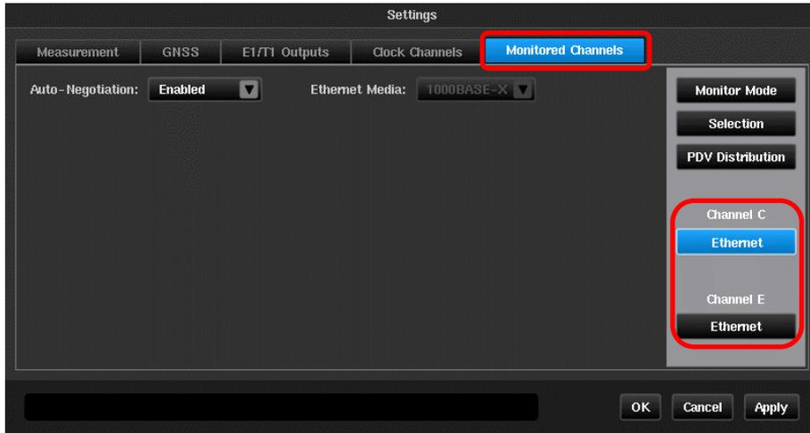
There is an Ethernet page for both channels used and these should be set to the same values. Electrical TAPs may require **Auto-Negotiation** to be **Enabled** while optical splitters generally require a fixed rate to be entered.
