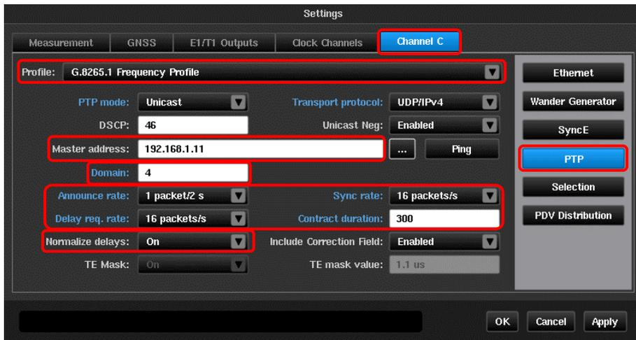
**NOTE:** Ensure the IP address of the Sentinel pseudo-slave is provisioned before going out into the field.
