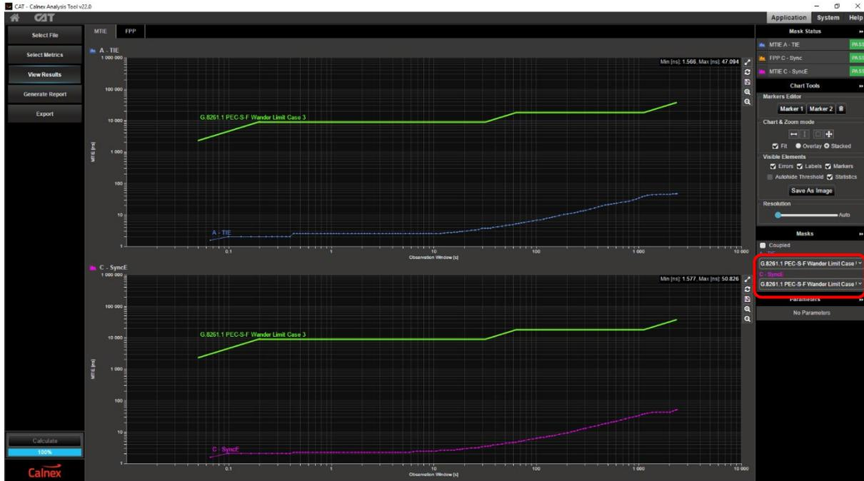
The FPP results can be viewed on the **FPP** tab. By default the parameters are set for the ITU-T G.8261.1 limits but can be adjusted if necessary. A summary of the Pass / Fail status of each metric is shown in the top right corner.
