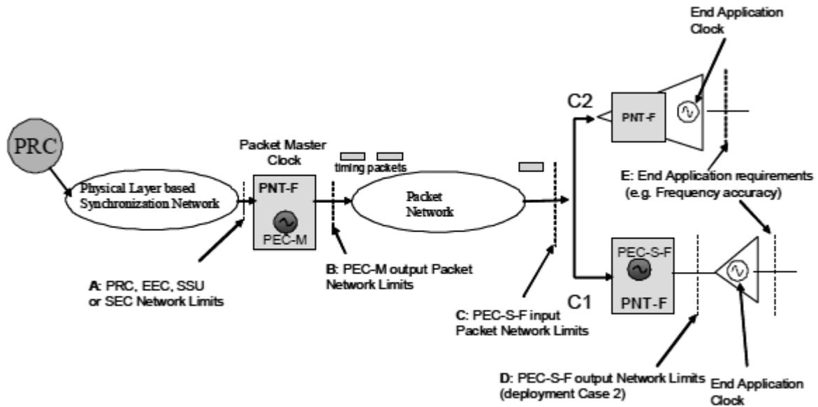
Network limits are specified at different level of reference points. At reference point C, the packet network limits are expressed in terms of the relevant PDV based metric as follows:
