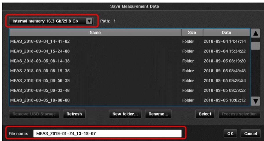
**NOTE:** For longer term measurements, it is always recommended to use external USB memory sticks to ensure sufficient storage space.
