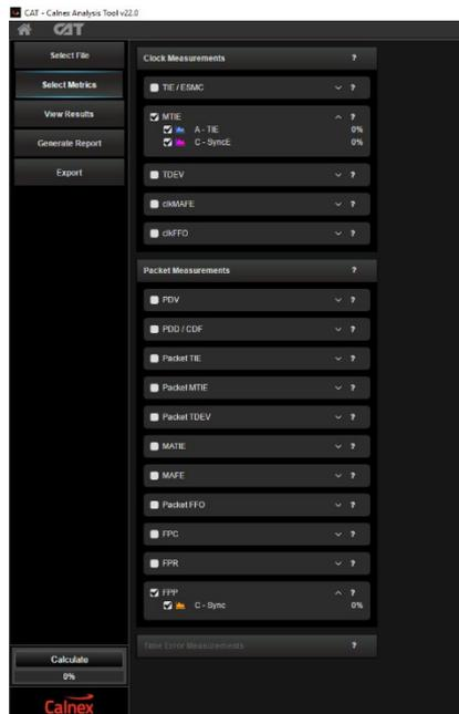
The clock measurements box should enable MTIE for the 10MHz recovered clock (A TIE) and SyncE recovered clock (C – SyncE) if that is being tested.
