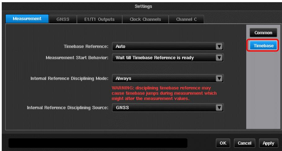
**NOTE:** From a cold start, it takes around 15 minutes for the internal Rubidium timebase to warm up. With the GNSS antenna connected, the GNSS receiver needs to lock to at least 3 satellites before it can output a valid reference to the Rubidium for disciplining. If less than 3 satellites are locked, the Rubidium will go into holdover.
