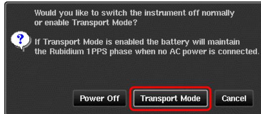
**NOTE:** Without mains power supply, the battery can keep the internal Rubidium powered for up to 3 hours. Once mains power is supplied again, the Rubidium will be powered by the main supply and the battery will start to re-charge.
