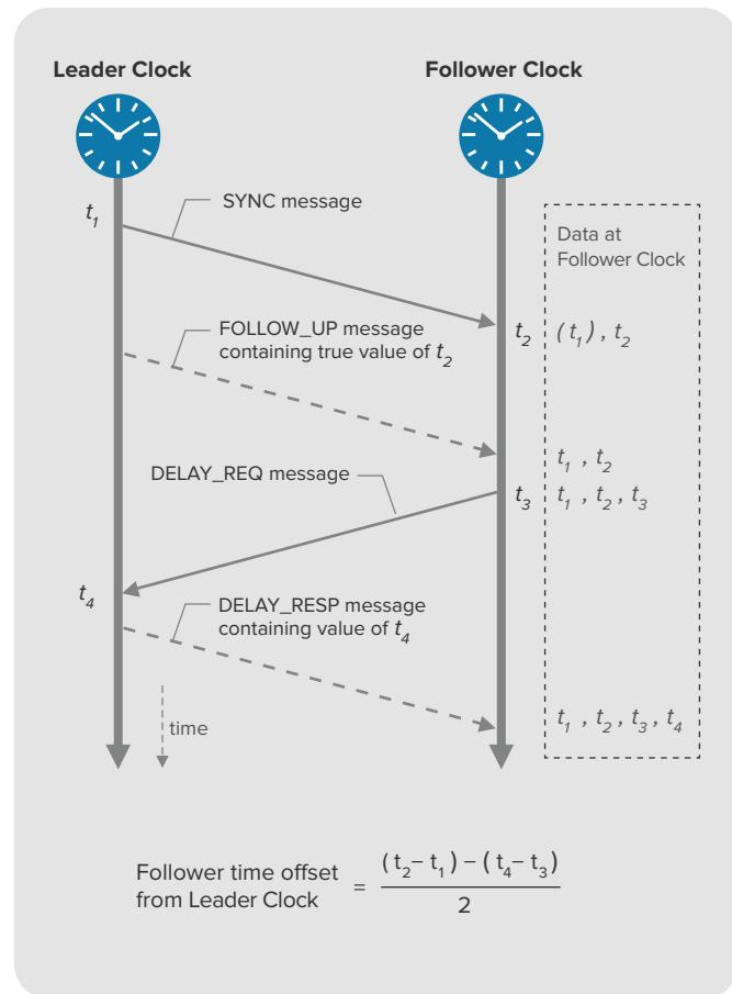
The time offset is then estimated using the assumption that the one-way network delay is half the round-trip delay and is used to correct the follower time base to align to the leader.
